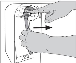
Keep the pump block pressed down with the finger and pull the pump out to the front. Simultaneously swivel the top of dispenser unit, to allow the pump to be removed forwards.
