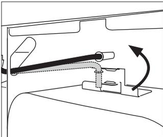
Turn the end of the outlet pipe 90° anticlockwise.
